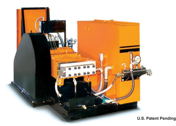
NLB's newest line of waterjetting units are built around the innovative model 125 convertible pump. This pump, with its quick-change, in-line fluid end design, has fewer parts for increased operating efficiency and simpler maintenance. And, it requires only a simple conversion kit to operate at pressures between 6,000 psi (414 bar) and 24,000 psi (1,680 bar).
