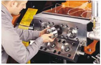
NLB's operator friendly pump designs make on-thejob maintenance and pressure conversions simple.
